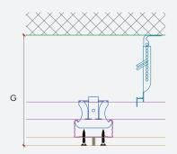
\* Is to be adjusted and fitted according to the exact length of the panel (please note that the size of the panels varies depending on the type of perforation).
